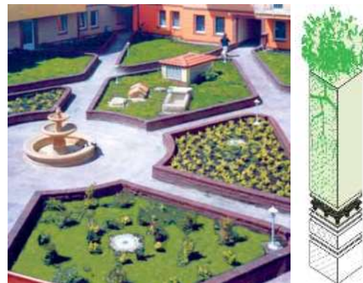
Fig. 5. Composition of an Intensive Green Roof [6].
