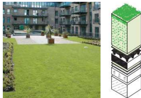
Fig. 4. Composition of a Semi Intensive Green Roof [6].
