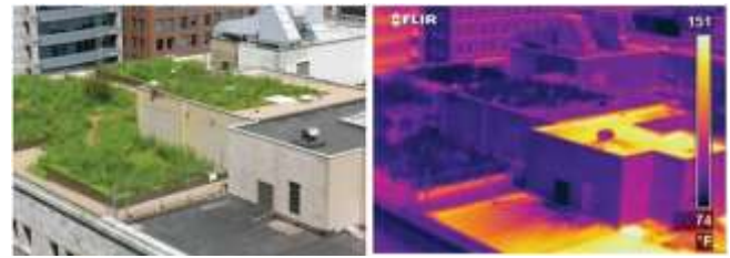
Fig. 8. Example of temperature differences between a green roof and a conventional roof [4].
