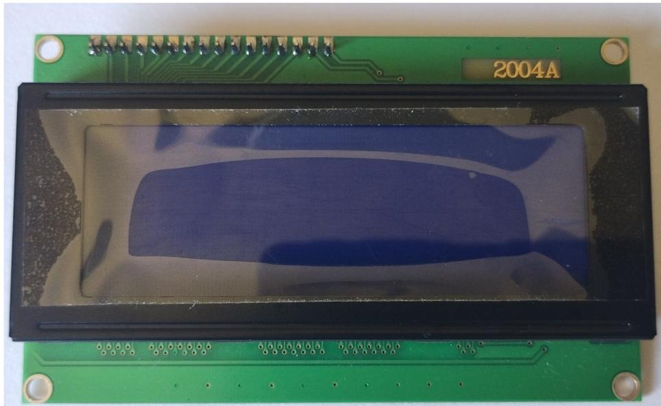
Figura 3.8: Display LCD 20x4.
