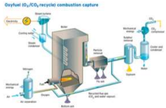
Figure 6: Simplified flowchart for an oxy-fuel power plant [5]
