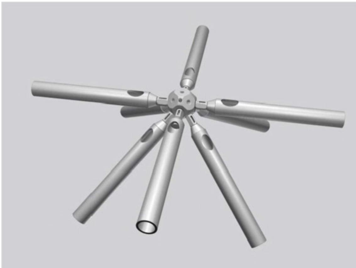
*Figura 94: Esquema Sistema Mero en un Nodo*
