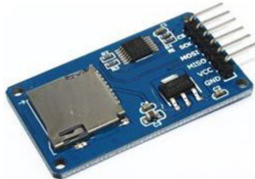
Fig. 1.17: SPI Micro SD Storage Micro SD TF Card Memory
