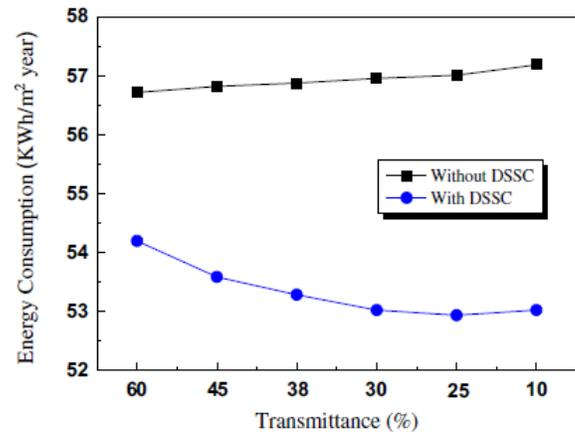
Fig. 8. Total energy consumption by year vs transparency with DSSC
