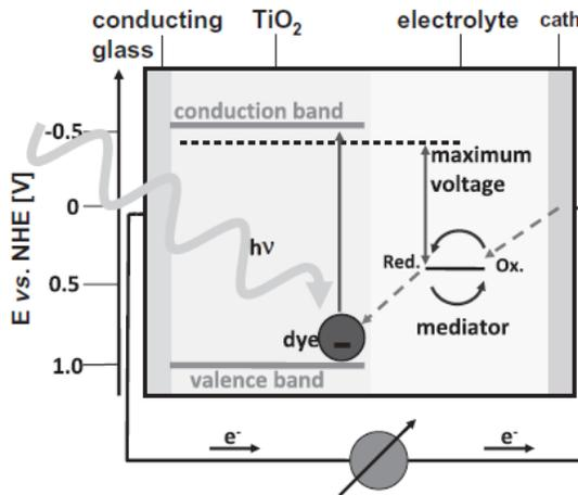
Fig. 3. DSSC Electrochemical process.
