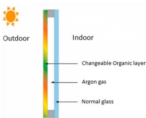
Fig. 9. Schematic representation of the COSW
