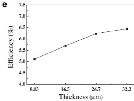
Fig. 5. Cell Efficiency vs Thickness of organic layer
