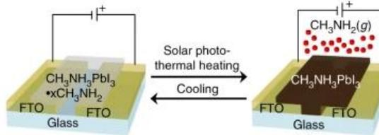
Fig. 10. Schematic representation of the chemical reaction
