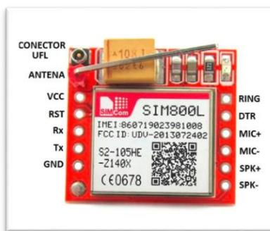
**Fig.2** “Módulo SIM800L”
