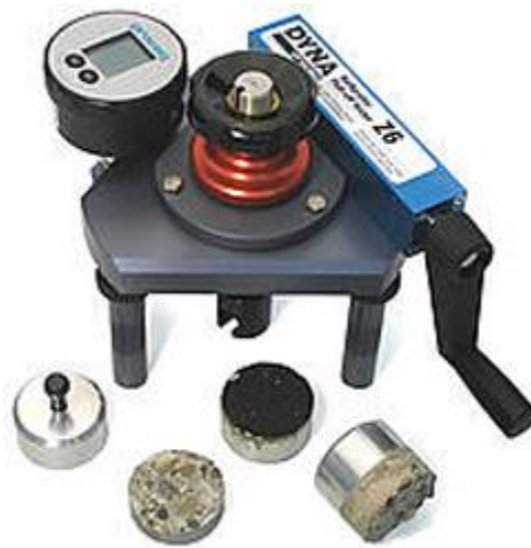
Figura B-6. Pull-off Test Method Fuente: www.capco.co.uk
