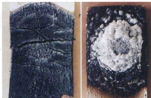
Figure 2. Left, panel without treatment and right, film of intumescent coating, both after the fire action.
