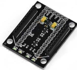
Imagen IV.26: XBee Explorer Regulated
