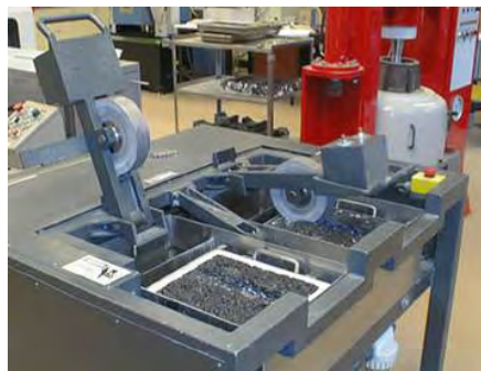
Figura III.3 Hamburgo Wheel Tracking Device (HWTD)
