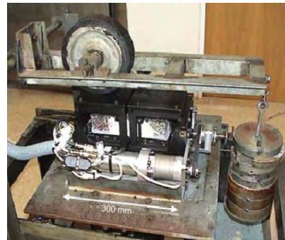
Figura III.1 Wheel Tracking Test (WRC)
