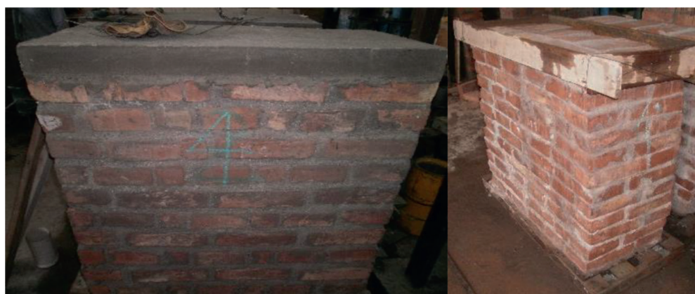
Figure 7. Preparation of masonry specimens [33].
