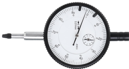
Fig. 1. Dial indicator with 0.01 mm resolution.
