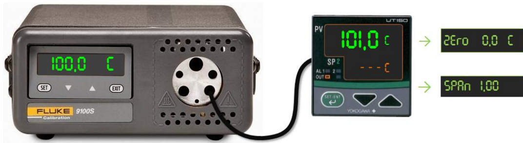
Figure 5. Simulating zero and span adjustments in a temperature controller
